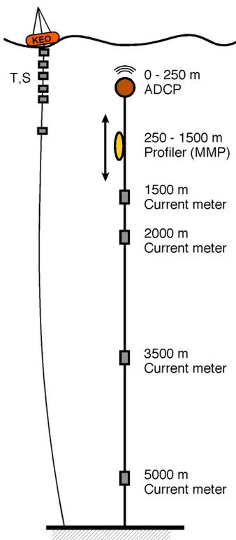
Figure 1: Schematic of a KESS subsurface mooring and of KEO (close to KESS-7)
