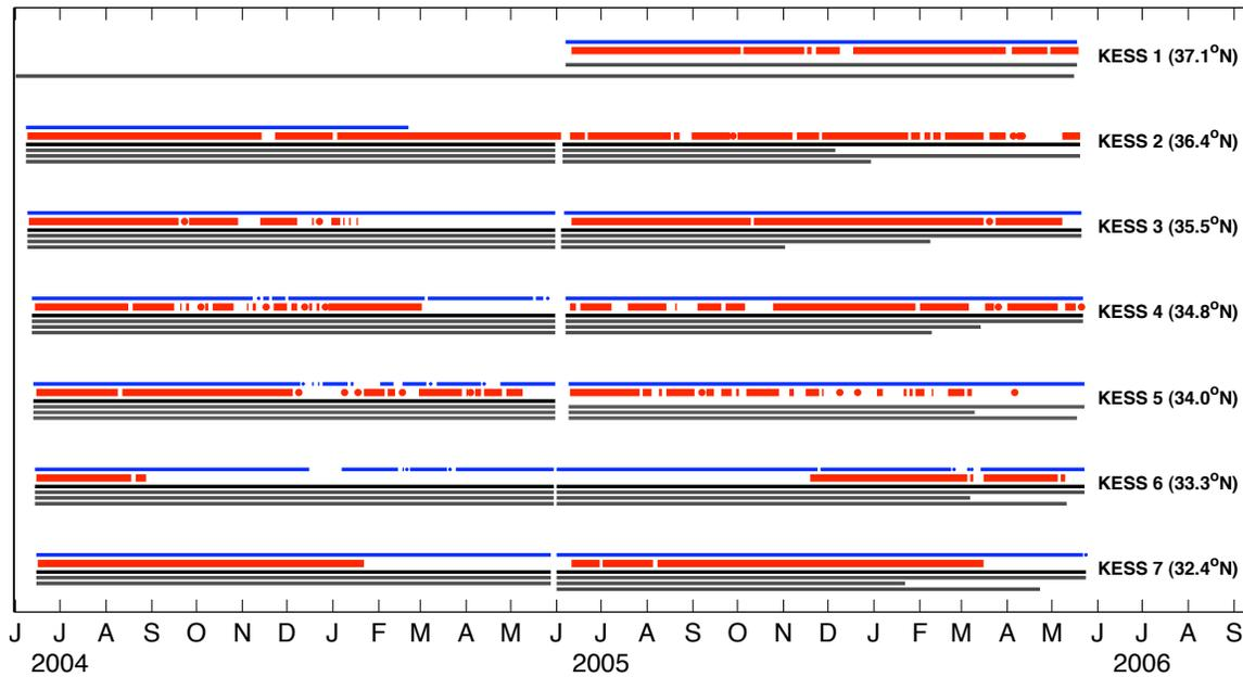
Figure 3: Data return was high from the sub-surface current measurements, but MMPs returned partial records. A line is plotted when measurements are good: ADCP (blue), MMP (red), and deep current and temperature measurements (VACM, black; RCM, gray). The turn-around cruise was in June 2005.
