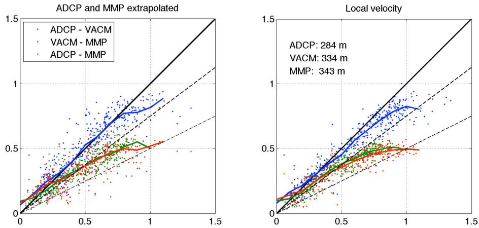
Figure 10: Comparison of the speed recorded by the ADCP, a VACM, and the MMP near 250 m during the first year at KESS-4. MMP and ADCP speeds are extrapolated to the depth of the VACM in (a) using an estimate of vertical shear, and closest data point is used in (b). Reference lines have slopes of 1, 4/3, and 2.
