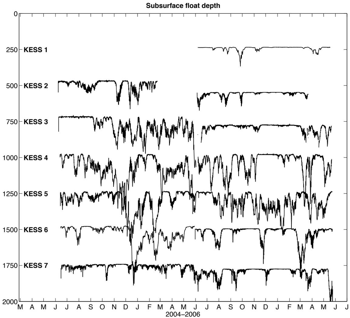
Figure 7: Time series of the depth of the ADCP at each mooring. The vertical axis is for KESS 1, and each subsequent mooring is offset by 250 m. Depths are obtained using the ADCP intensity profiles and the MMP pressure.
