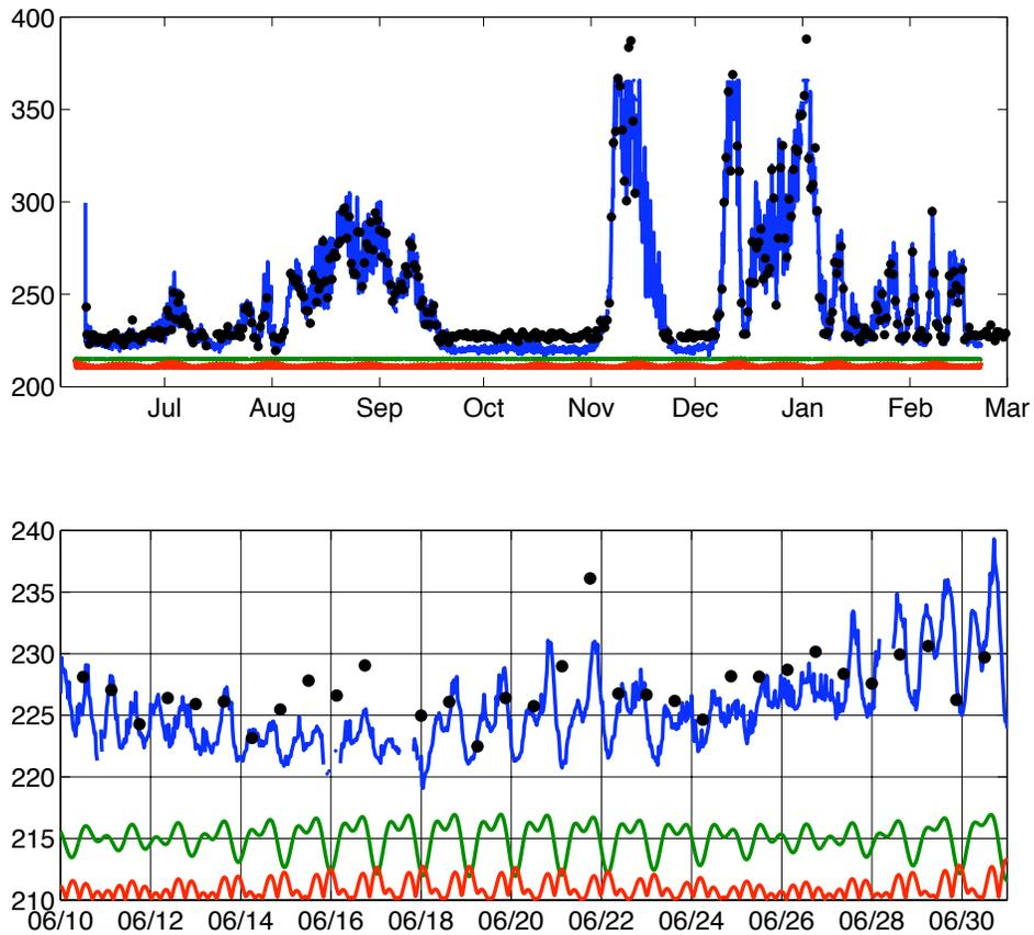
Figure 6: Distance between the surface and the ADCP, for KESS 2, during the first year (2004-2005). The best estimate from the intensity profiles is shown in blue, the minimum depth of the MMP (-20 m) is in black. The TPXO.6 barotropic tide elevation ( $\times 5$  in (b) ) is shown in green, and the magnitude of barotropic currents in red. (b) shows a close-up.
