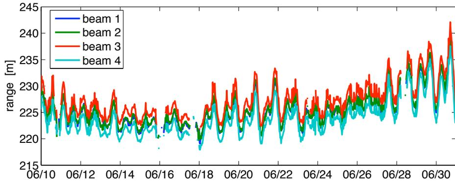
Figure 5: Ranges from the ADCP to the surface inferred from intensity profiles, from KESS 2. Each of the 4 beams is shown for a period of about 3 weeks in June 2004.
