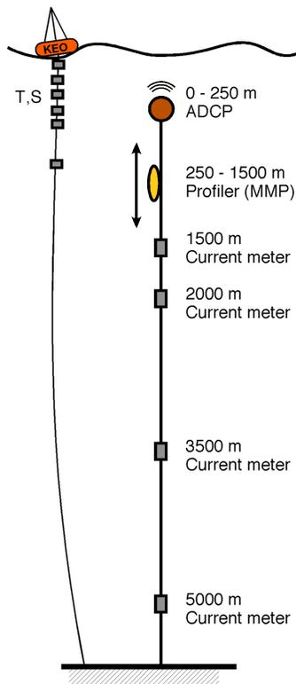
Figure 1: Schematic of a KESS subsurface mooring and of KEO (close to KESS-7)
