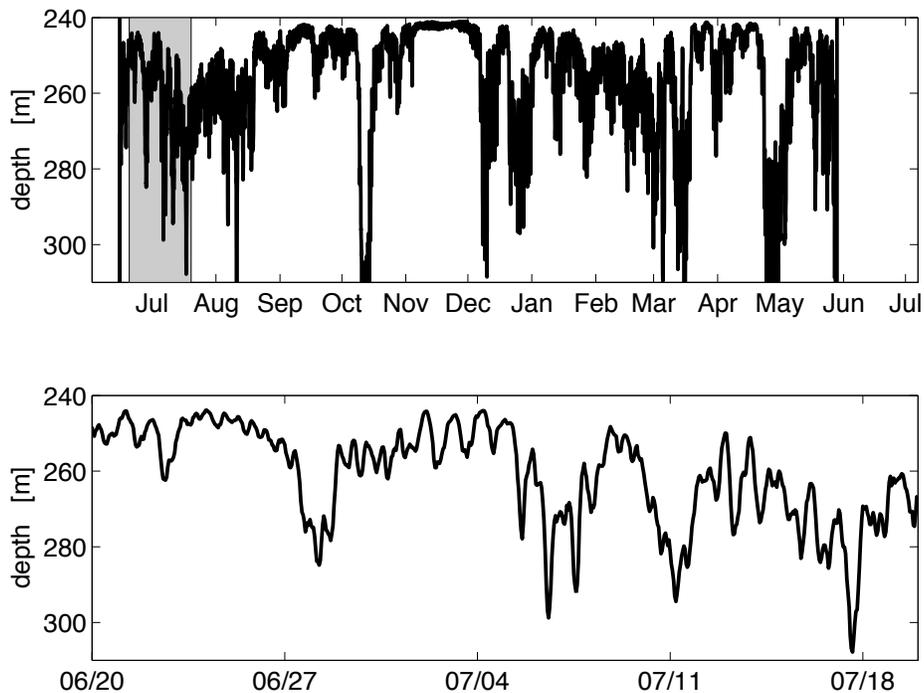
Figure 4: Depth of the ADCP at KESS 7 during the first year deployment (2004-2005). Data obtained from the PMEL TP recorder. The entire time series is shown in (a), and a close-up (indicated by the gray area) in (b). Tidal signal is evident.
